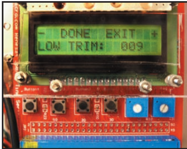
Photo 2 —This is an example of screen output for the servo trim settings. In this case, the user is setting the servo’s maximum return angle.
