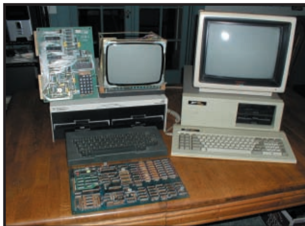
Photo 1 —Personal computing in the 1980s. On the left is my CP/M machine, which is based on the J.B. Ferguson "Big Board." A spare CPU board sits in front of the keyboard. On the right is the Zenith Data Systems PC (an IBM PC/XT clone) that replaced it. To the left of the CP/M monitor is a KIM-1 board, a 6502-based single-board "system" that was popular with hobbyists. It includes a hex keypad and display, along with a monitor program in PROM to operate it.
