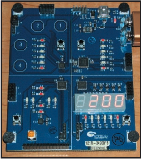
Photo 2—With four PSoCs and all the trimmings (e.g., an accelerometer, USB and LCD interfaces, and LEDs), the Cypress World Tour demo board has something for everyone.
