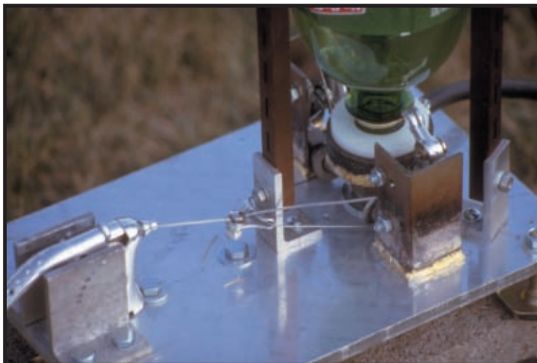
Photo 1 —Combine some bike parts with a soda bottle, add some parallel-port electronics, stir in a bit of firmware, and we had the single most popular project ever: The Circuit Cellar Strategic Defense Initiative . Two hundred issues later, we still get e-mails!
