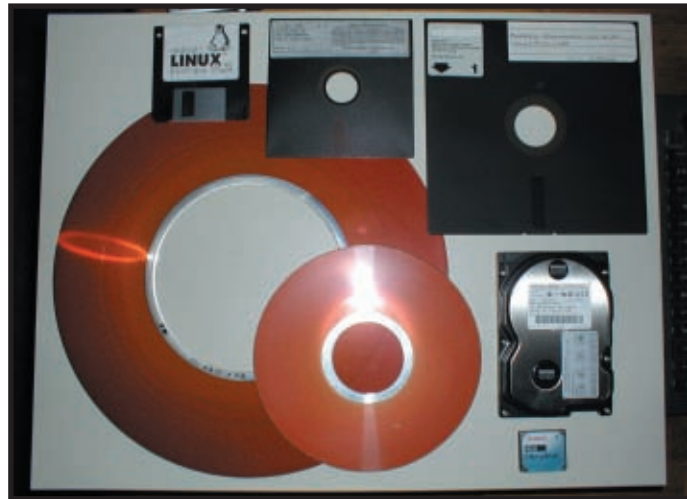
Photo 2 —This collection of disks (sitting on top of the CPM disk drive cabinet shown in Photo 1) shows the advances in magnetic disk storage. From left to right across the bottom are a 14" platter and an 8" platter. The former shows evidence of a head crash about halfway out. To the right of these is the ubiquitous 3.5" hard drive, which comes in capacities of hundreds of gigabytes these days. Below that is a 4-GB "Microdrive" that fits in a compact flash memory slot. From right to left across the top are 8", 5.25", and 3.5" floppy disks.
