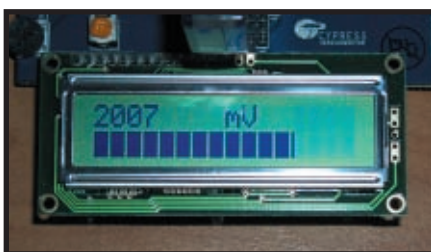
Photo 4—The LCD bar graph in action. Note that the function also supports four-line displays, a feature that allows two parameters and bar graphs to be displayed simultaneously.
